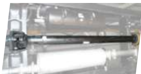
LFL PROPELLER SHAFT FOR MAINTENANCE FREE OPERATIONS
