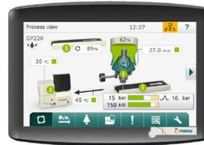
Automatic **crushing optimization** by feed-rate control, based on material level and crusher's load conditions
