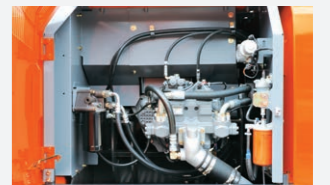
Grouped remote filters and inspection points
