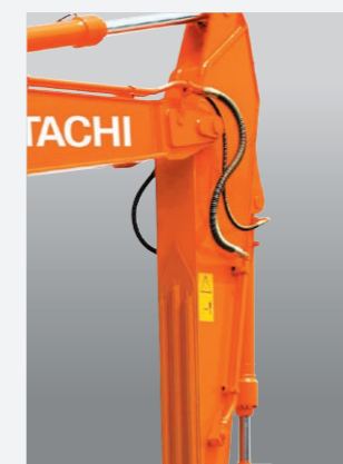
Attachment basic piping
