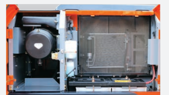
Utility space and radiators
