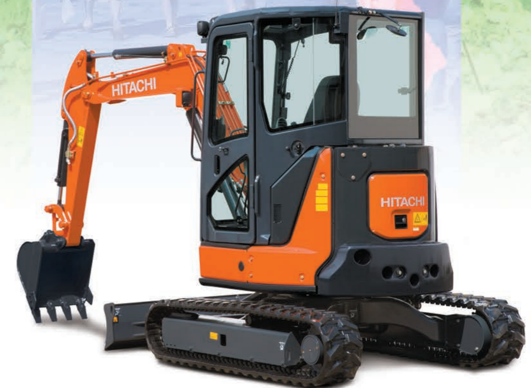
Shown equipped with 1.52 m arm, additional counterweight, cab and extra piping and as optional items.
