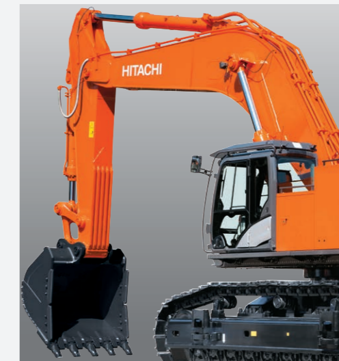
Enhancements of boom & arm with rock bucket (ZX870H-5G / ZX870LCH-5G)
