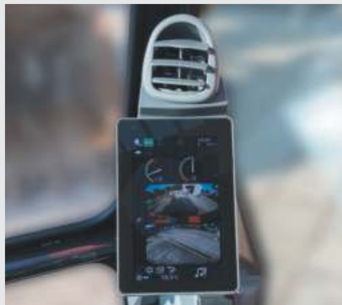
Low-reflective color 8" monitor, 42% larger display compared to ZX-5G series. Easier to view and navigate. Bluetooth® and USB power supply available.
