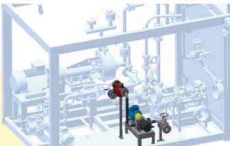
There are two options for kerosene dosing system; - High flow rate (%25-60) to produce cut-back (MC). - Low flow rate (%3-10) for softening the bitumen.
