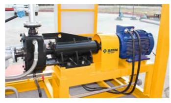
emulFALT's **emulMILL** with its **adjustable milling gap** provides <6 µm particle size and guarantees the best quality of final product even with low penetration bitumen. Thermal oil or electrically heated mill is suitable for the production of both anionic and cationic emulsions and also modified bitumen emulsions.
