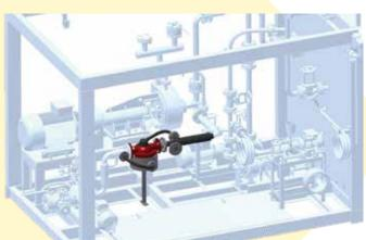
Bitumen mass flowmeter to produce high-quality emulsion. Thanks to bitumen flowmeter; the actual amount of bitumen flow, total amount and other parameters can be checked and adjusted properly.
