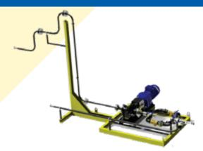
Latex Dosing System is an external part of the emulsion plant that feeds the plant with latex through a dosing pump which is equipped with an inverter for perfect dosing rates. Latex Dosing System can be easily positioned according to worksite layout thanks to its flexible hoses and compact size. Dosing rate can be adjusted in accordance with the recipe.
