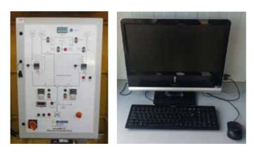
Control system of the emulFALT is **manual as a standard.** However, PLC & SCADA control system with embedded touch screen computer on the control panel or control cabin with PC options are available.
